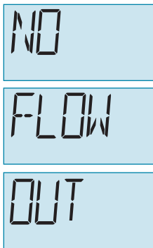
Figure 3-5 NO FLOW OUT Alarm
